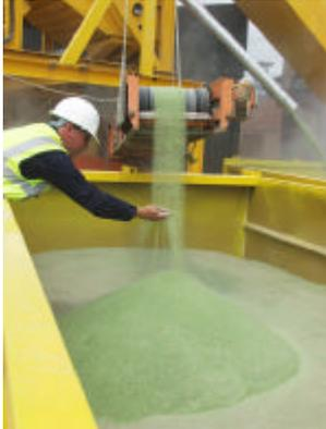
The purpose of glass crushing equipment is to reduce the glass containers into fragments of glass of consistent particle shape and size. The usual measure of particle size is through a sieve test, where the glass is sorted into those fragments small enough to pass through a sieve and those fragments retained on the sieve because they are too large to pass through the sieve. Standard sieve sizes can be found in Appendix 1.
