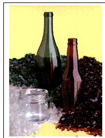
When recycling glass back into these markets care must be taken to use only glass which has a similar composition to the primary feedstock, this will help prevent inclusions and other anomalies arising from feedstocks with varying melting points etc.
