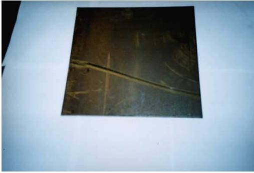
*Figure 4: Oxidised plate before blasting*
