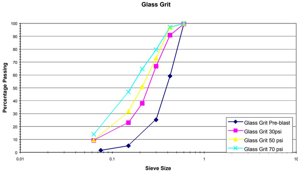
It can be seen from the above graph, that the higher the pressure, the greater the breakdown rate is for the glass grit which is as expected, with a higher percentage of particles passing the same sieve size.
