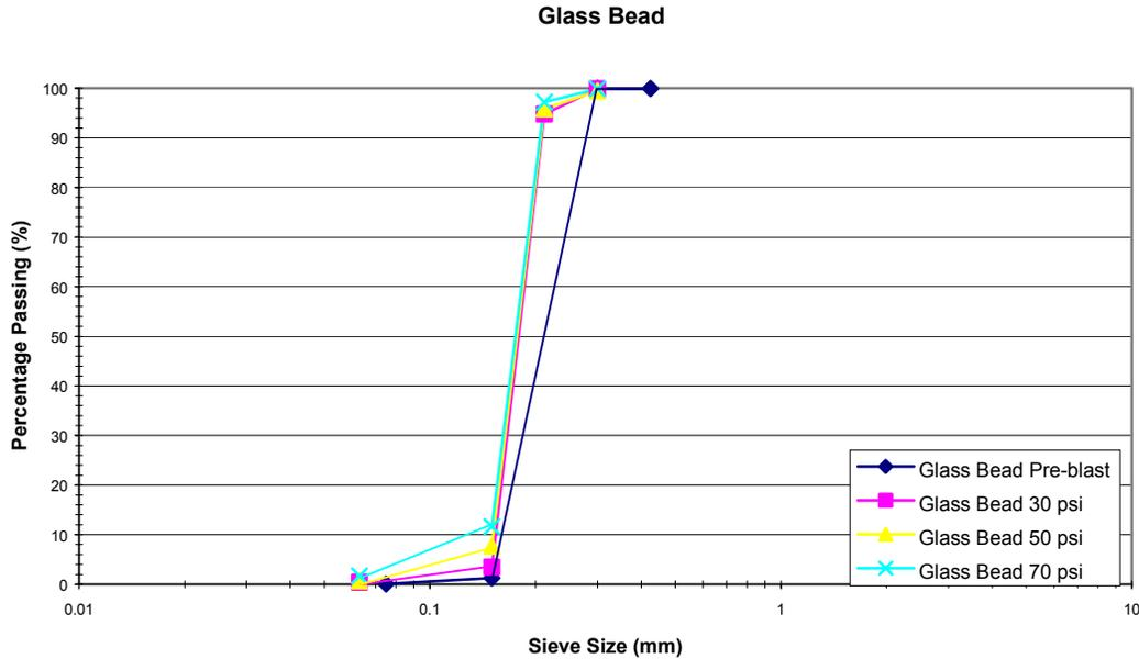
As expected for the glass bead, it appears to have less initial breakdown than either the copper slag or glass grit, and that there is only a marginal increase in breakdown rate with increase in pressure.
