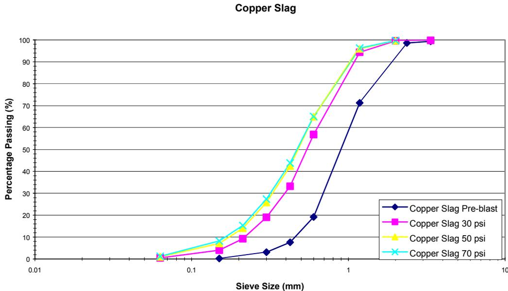
The above graph shows that the initial breakdown is high, and that the change in pressure thereafter only has a marginal effect on the breakdown of the abrasive. The graph shows only a small percentage of fines, however this was of a dirty nature and had the appearance of a dark chalk-like residue.
