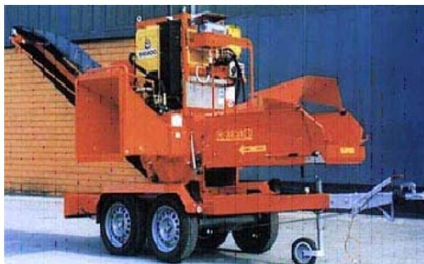
ARCO currently process around 150 – 200 tonnes of glass per annum on the island, and find this piece of equipment satisfactory for Arran's needs, as it is also used in the winter to shred cardboard for animal bedding. However, the glass is extremely hard on the hammers and they require to be replaced after only 20 tonnes of processing. ARCO are now using second-hand hammers which have reduced maintenance costs from £400 to approximately £250 per replacement.
