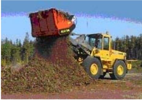
drums rotate in the same direction. The hydraulic power from the base machine is transferred via hydraulic hoses to the hydraulic motor of the screener/crusher. The hydraulic motor then transfers the power to the drums via chains and chain wheels. The screened and crushed material flows through the crushing and screening drums when the blades scoop the material through the drums.
