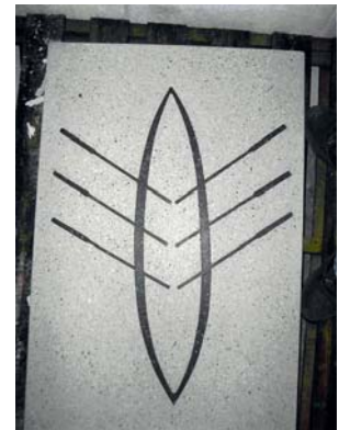
Eniroglass Tile made with recycled glass
